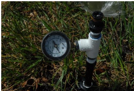
Test working water pressure at the first and last sprinkler with a pressure tee and gauge.
